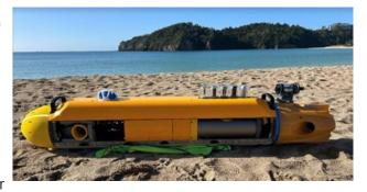
Vehicle (AUV) capable of operating over complex regions of seafloor and collecting high resolution benthic imagery.
