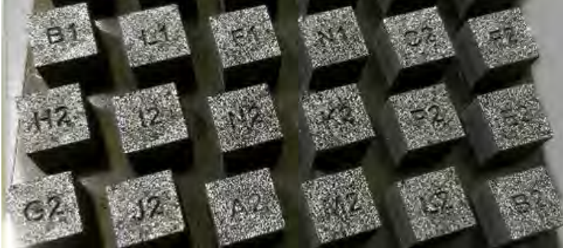
First Batch of pure Nb specimens produced on the laser powder bed platform (Concept Laser MLab) in SMH
