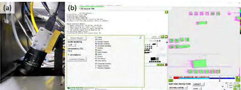
Fig. (a) Off-axis high resolution monochrome camera installed to view the printed surface of the LPBF system. (b) The Peregrine AI software interface, displaying real-time semantic segmentation of printed components, soot, and other defect classes.
