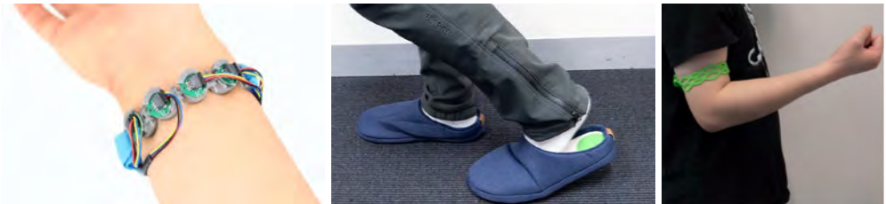
3D printed sensors - left to right- sensor bracelet, in-sole sensor for gait analysis and sensor band to track arm movements.
